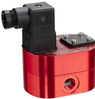
The flow meter measures the moving dosing volume of liquids according to the gearwheel principle. A pair of gears fitted very precisely into the housing forms the measuring mechanism. The rotation of the measuring mechanism is detected tooth by tooth without contact by a signal pickup system and converted into digital pulses.
