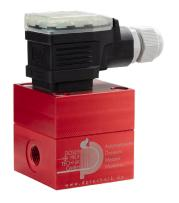
The flow meter measures the moving dosing volume of liquids according to the gearwheel principle. A pair of gears fitted very precisely into the housing forms the measuring mechanism. The rotation of the measuring mechanism is detected tooth by tooth without contact by a signal pickup system and converted into digital pulses.
