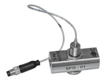
The flow transmitter is used to monitor the metering process and is located between the metering and dispensing points. The flow of the metered medium is detected by a pistonstroke monitoring by means of a proximity switch.
